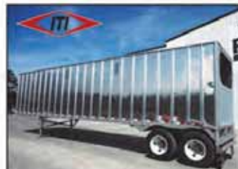
Innovative 42' x 102' x 13'6" Closed Top Chip Trailer
